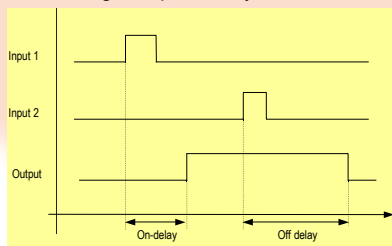
Fig. 6: Example for one effect of the pulse shaper stage
